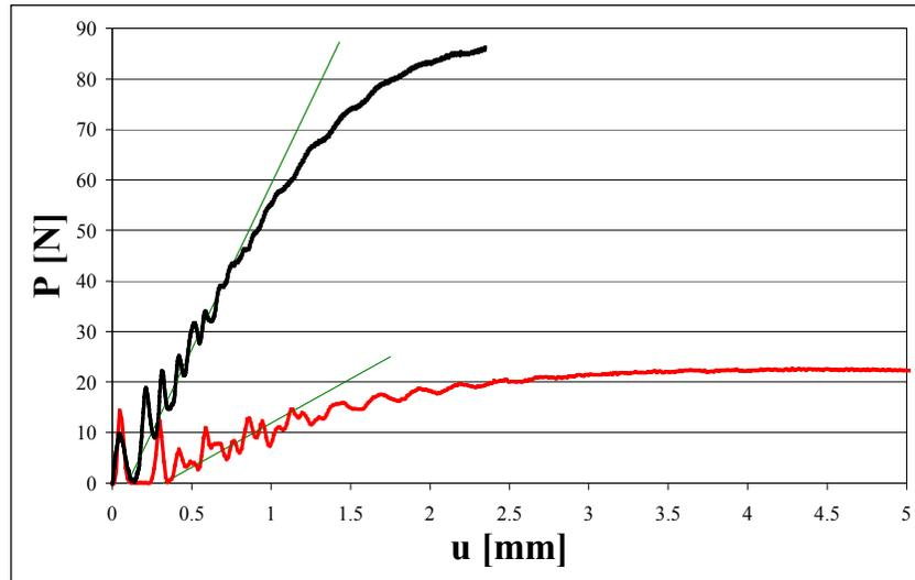
Fig. 4: Load vs displacement curves measured for blunt (red) and sharp (black) notched specimens
