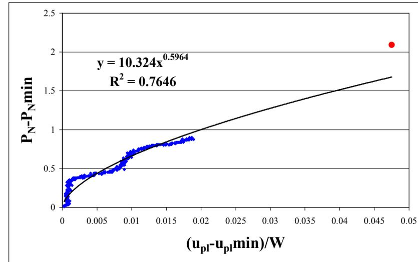
Fig. 6: Construction of the "material key curve"
