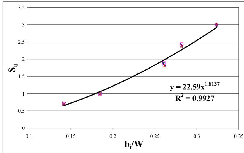
Fig.3: The separation parameter vs  $b_i/W$  for blunt notched specimens
