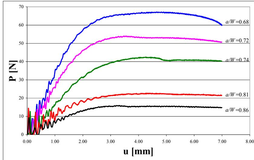
Fig.1: Load vs displacement traces of blunt notched specimens
