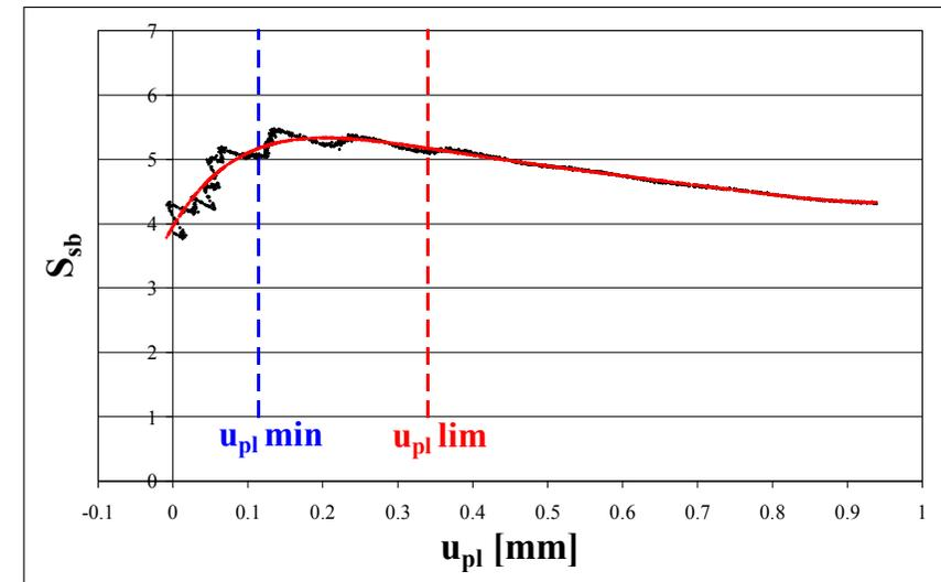
Fig. 5: The separation parameter  $S_{sb}$  vs plastic displacement for the sharp notched specimen
