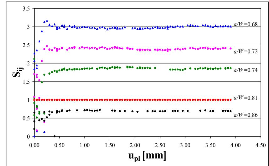
Fig.2: The separation parameter vs plastic displacement of blunt notched specimens
