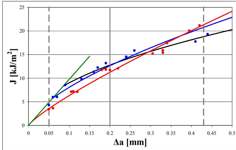
Fig. 7: Comparison among  $J_R$  curves determined using the different J-testing procedures (separation criterion - black, "reduced velocity" - blue, "striker stop" - red)
