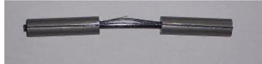
*Fig.8: Typical appearance as brush of a fractured specimen*
