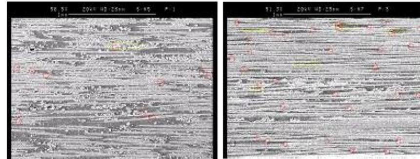
Fig.5a: Enlargement of a section of the specimen loaded until  $\sigma/S_u=0.24$ . Number of fibre cracks is about 10; number of matrix cracks is about 4, number of interface cracks is about 1, with length 0.35mm
