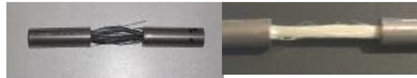
Fig.3a: Black specimen fractured
