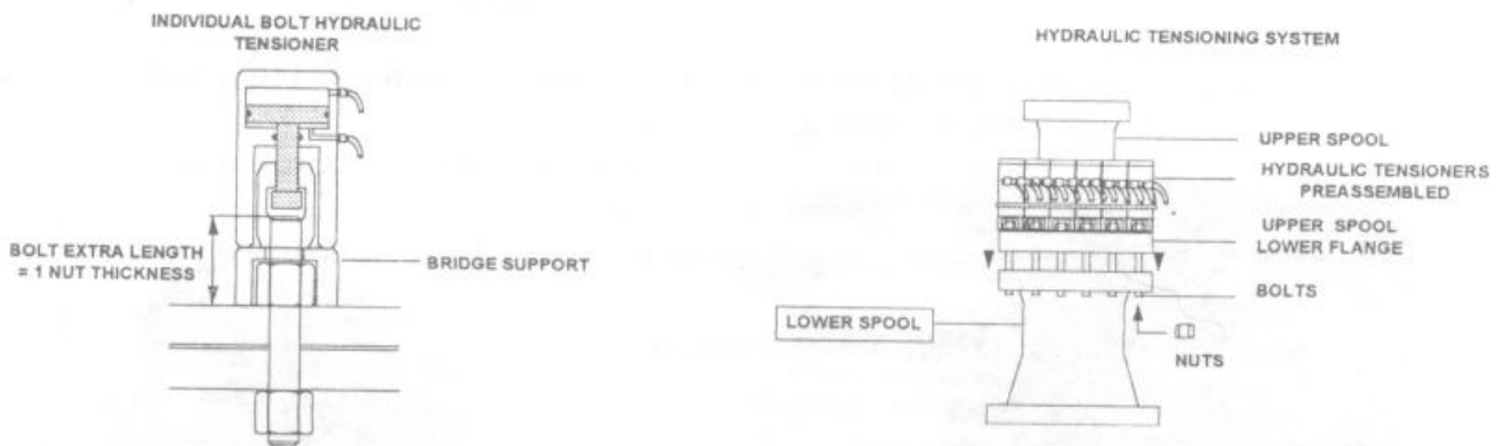
Fig.4 - Hydraulic tensioning device
