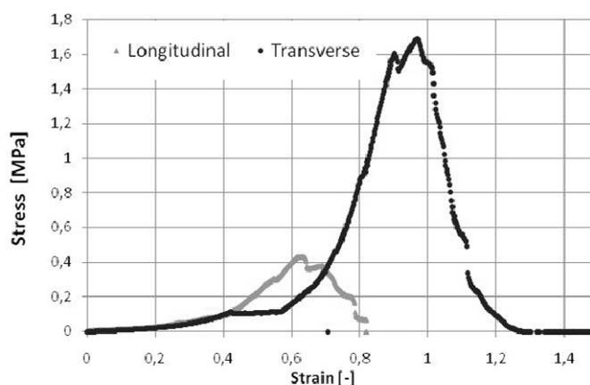
Figure 2: Typical stress-strain curves obtained for pig coronary arteries, longitudinal and transverse direction.
