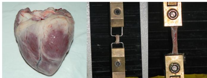
Figure 1: Heart with marked coronary artery; samples mounted in strength machine grips.
