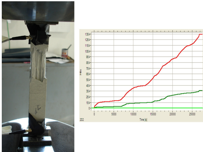
Figure 5: Broken specimen and AE signal associated to the fatigue test
