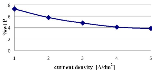
Figure 1: Influence of current density on contents of P in electrodeposited alloys.
