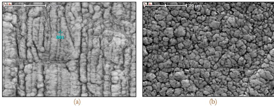
Figure 2: SEM images of surface of Co-P alloy deposited on copper (a) – pulse current method (waveform 1); deposition pulse time 10ms at current density of 6A/dm<sup>2</sup>, rest pulse time 10ms at current density of 0 A/dm<sup>2</sup>, (b) – constant current method, current density 3A/dm<sup>2</sup>.
