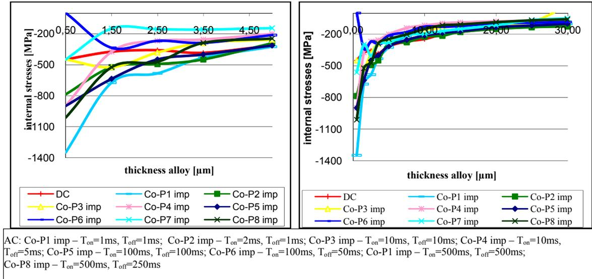
Figure 2: Influence of deposited by pulse current methods on internal stresses during deposited of the first 5  $\mu m$  of alloy
