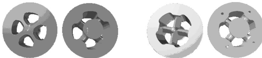
Figure 4: Geometry of the porthole die: standard (left) and blade (right).
