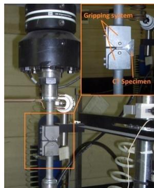
Figure 2: Gripping system for the application of a compression force at the specimen.
