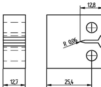
Figure 1: Shape and dimension of a fatigue crack propagation specimen.
