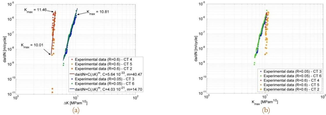
Figure 5: FCG rate curves in terms of: a)  $\Delta K$ ; b)  $K_{max}$
