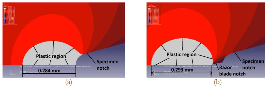
Figure 4: FE results in terms of Von Mises stresses at the specimen notch: a) original; b) after razor blade polishing technique.
