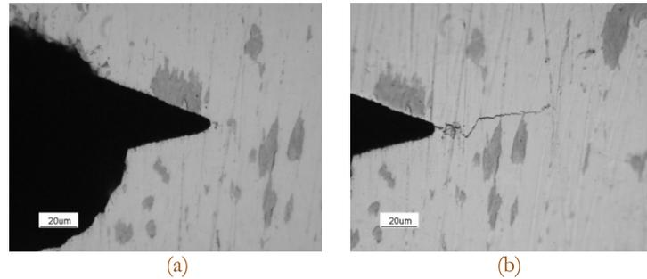
Figure 3: Notch of the specimen: a) after razor blade polishing technique, b) pre-crack obtained after compression pre-cracking procedure.
