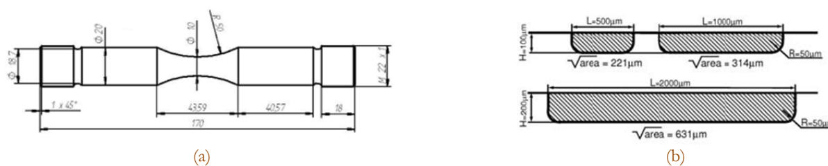
Figure 1: Out-of phase fatigue tests: a) bearing steel specimen geometry, b) micro-notches used
