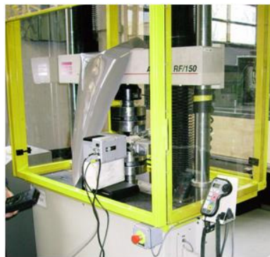
Figure 1: Testing set up (tensile tests and thermal analyses).
