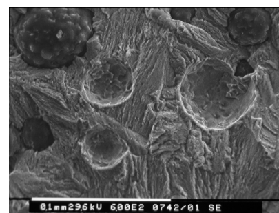
Figura 35: DCI perlite ( R = 0.1 , \Delta K = 16 \text{ MPa}\sqrt{\text{m}} ).
