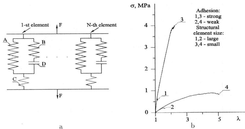
Figure 2 A set of structural elements (a) employing to qualitatively model the loading curves of an elastomer composite (b).
