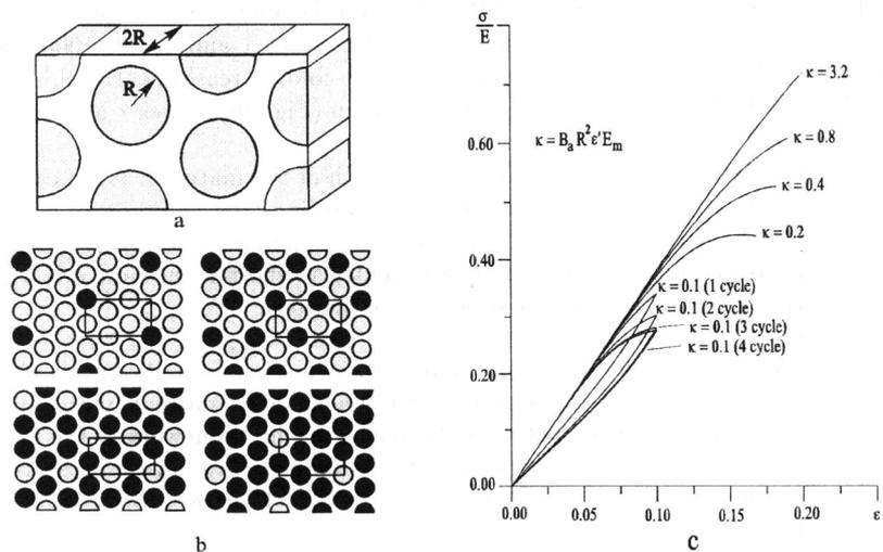
Figure 1 Schematic quarter of a periodical cell (a) being used to calculate damage evolution (b) and loading curves (c) for an elastomer composite.
