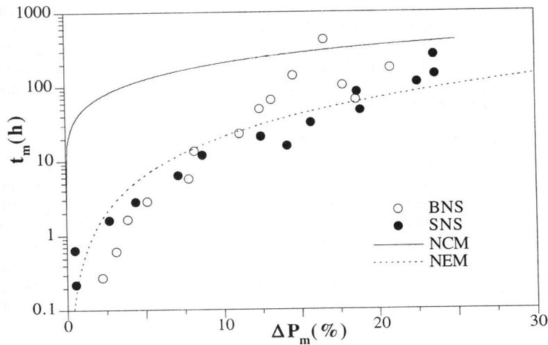
Figure 1 Loss of mechanical resistance versus embrittlement time for notched specimens of 316L steel stressed while hydrogen charged by cathodic polarization
