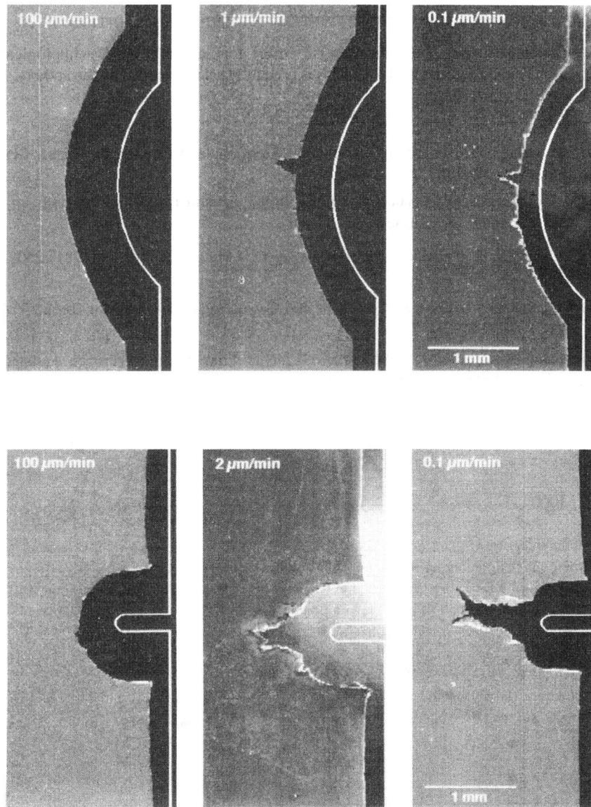
Figure 2 Notch profiles at maximum load of blunt (top) and sharp (bottom) notched specimens tensile tested at the indicated extension rate with simultaneous hydrogen charging (white lines show the shape and position of the original profiles).
