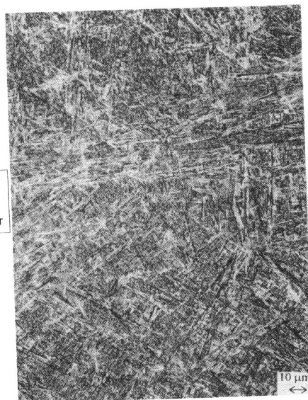
Figure 4. Weld metal microstructure EBW6B
