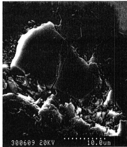
Figure 4. 10^4 cycles at 29.4 \pm 14.7 N at edge of contact zone.
