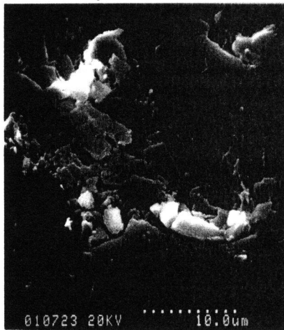
Figure 3. 1000 cycles at 38.8 \pm 20.6 N at edge of contact zone
