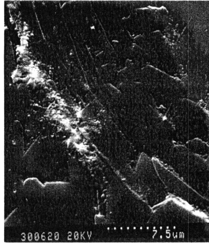
Figure 2. Specimen tested for 5000 cycles at 29.4 \pm 14.7 N. The contact zone is towards the right hand side of the figure.
