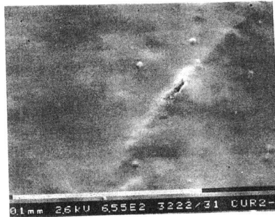
Figure 3 Micro-crack of 15 μm followed by PSB after 1000 cycles for \Delta\epsilon_T/2 = 8 \cdot 10^{-4} .
