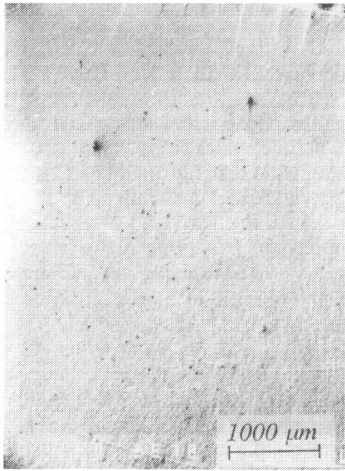
Fig. 5 Coaxial arc curves in the overload affected zone, 18Cr-9Ni steel
