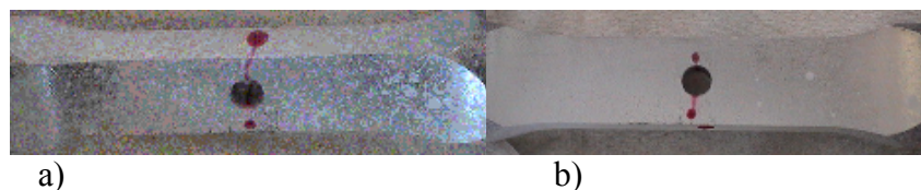
Figure 7. Liquid penetrant control; a) frontal-lateral, b) posterior (0.2mm,0.15% ).
