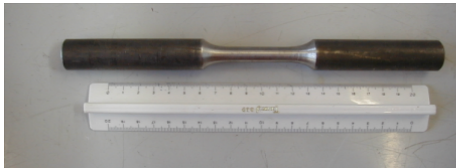
Figure 3. Actual specimen adopted for material testing.
