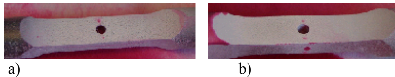
Figure10. Penetrant liquid on the posterior part of two specimens with slit 0.6mm a) \epsilon=0.2\% ; b) \epsilon=0.15\% .
