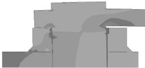
Figure 7. Bending stress due to the cylinder pressure of the wall of the ring.
