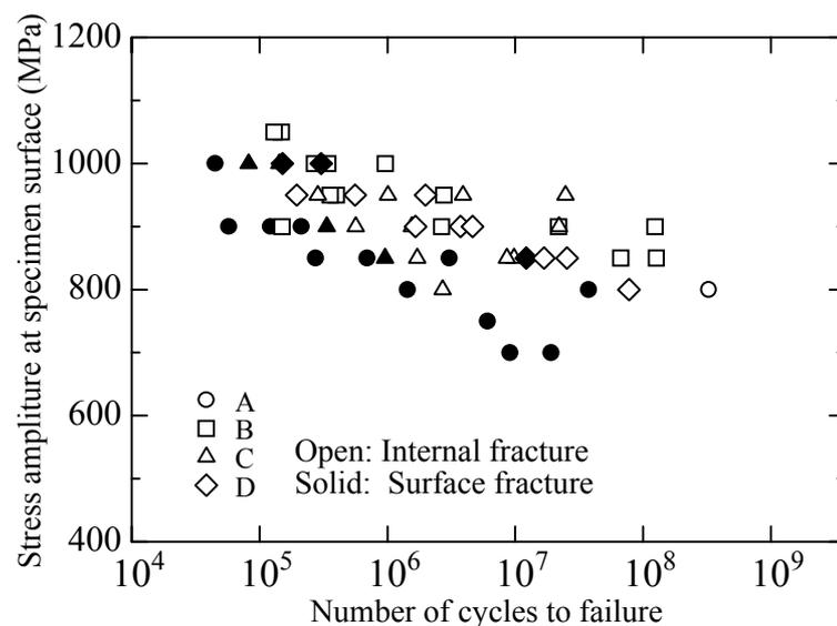
Figure 2. S-N plots where stress amplitude indicates one at specimen surface.
