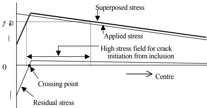
Figure 7. Stress distribution of bending specimen with compressive residual stress underneath the surface.
