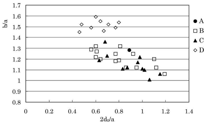
Figure 8. Relationship between  $2d_0/a$  and eccentricity of fish eye  $b/a$ .
