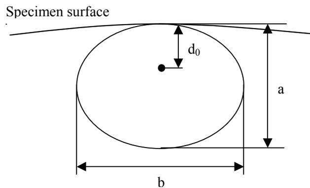
Figure 5. Definitions of parameters  $d_0$ ,  $a$  and  $b$  indicating the configuration of fish eye.
