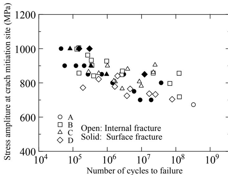
Figure 9. S-N plots where stress amplitude means one at crack initiation site.
