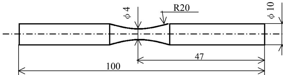
Figure 1. Profile of fatigue test specimen (in mm).
