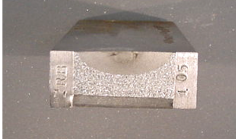
Figure 7 (b). Photograph displaying the actual shape of a thumbnail crack investigated.
