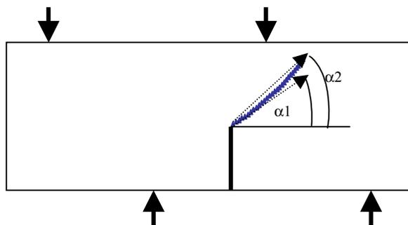
Figure 4. Angles determination  $\alpha_1$  and  $\alpha_2$ .
