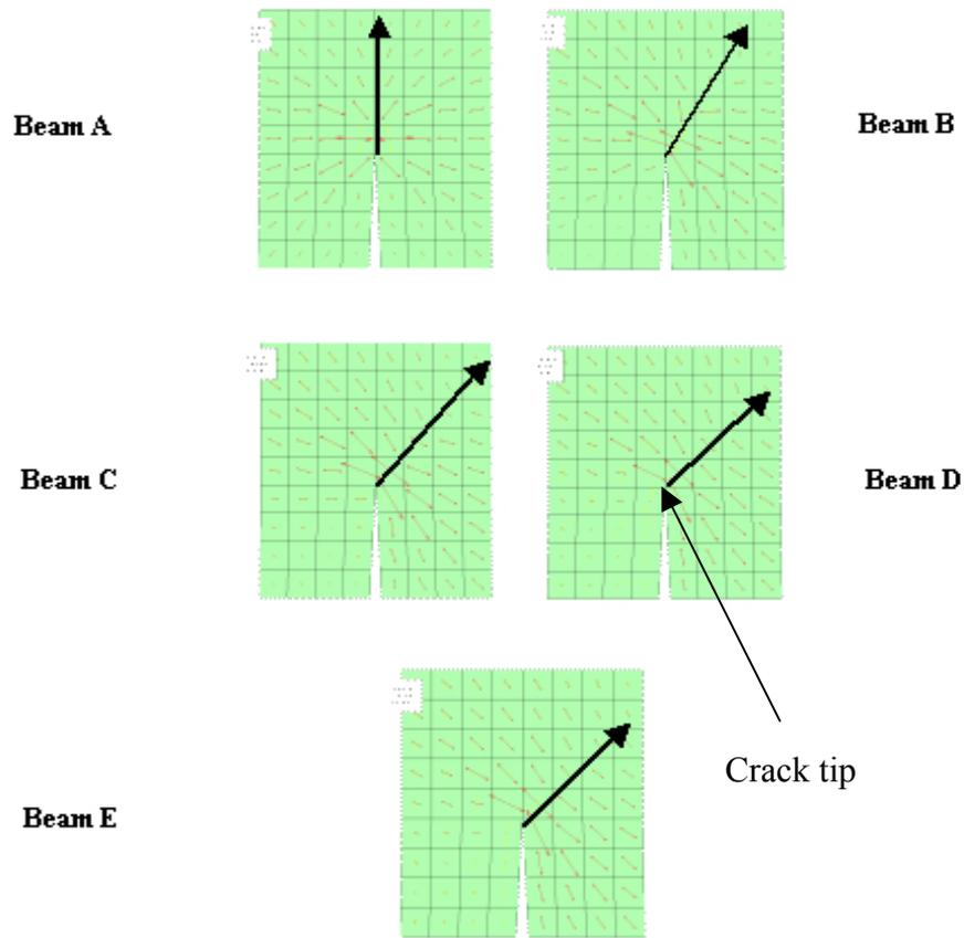
Figure 5. Estimation of the crack growth direction.
