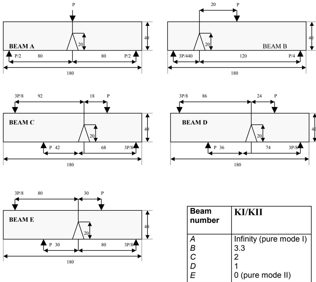
Figure 1. Tests and loadings (dimensions in mm.).
