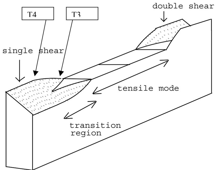
Figure 1. Drawing of the development of shear lips in a constant load amplitude test. At T3 the shear lips start, at T4 the surface is complete slanted.
