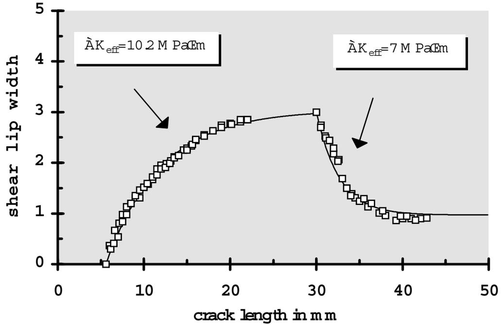
Figure 4. Shear lip width growth and shear lip width shrinkage.
