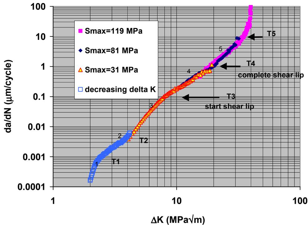
Figure 3. Experimental fatigue crack growth rate results for AA 5083
