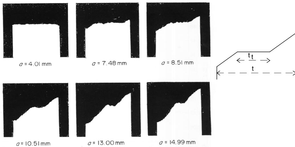
Figure 2. Transverse sections at increasing crack lengths.
