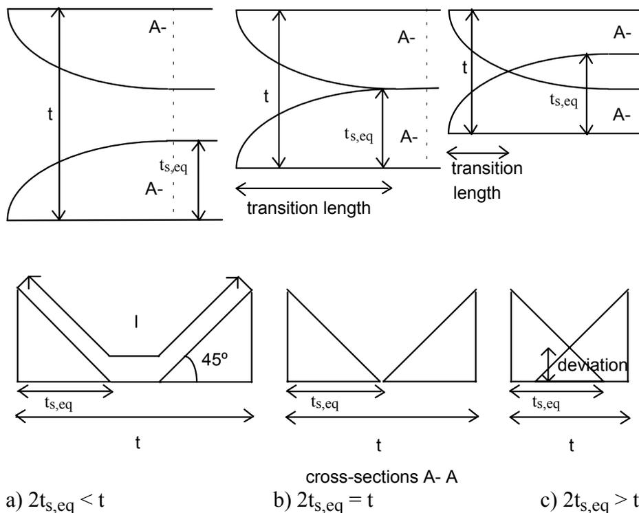
Figure 5. Double shear lip width development in a constant  $\Delta K_{eff}$  test.
