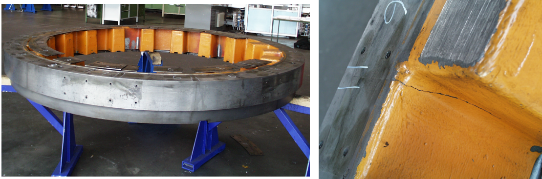
Figure 6. Shutter ring of a hydraulic press with detailed view on the crack propagation
