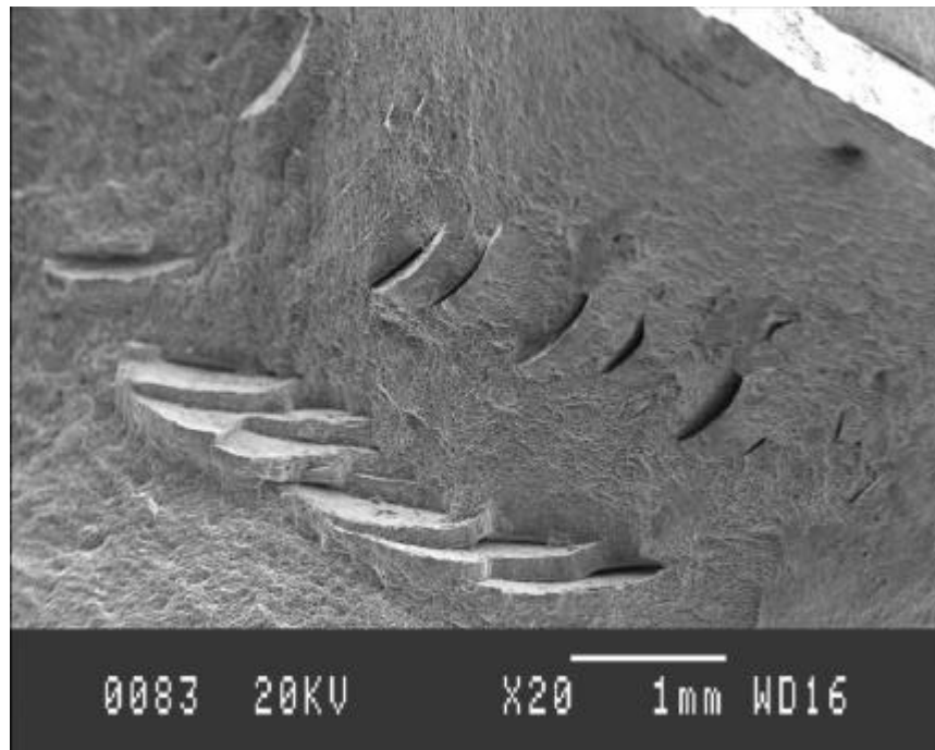
Figure 10. Planar facets on the fast fracture region of a tension fatigue specimen.
