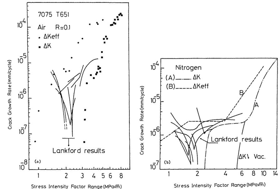
Fig. 11 Small cracks compared to long crack behaviour for the 7075 T651 alloy.
