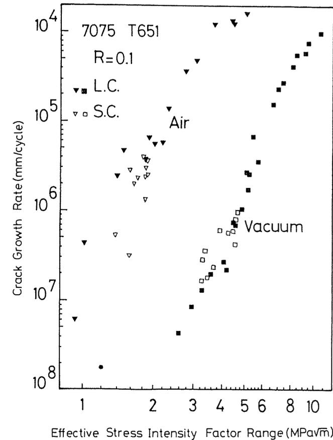
Fig 9 Crack growth rate versus  $\Delta K_{eff}$  for small and long cracks in air and vacuum; 7075 T651 alloy
