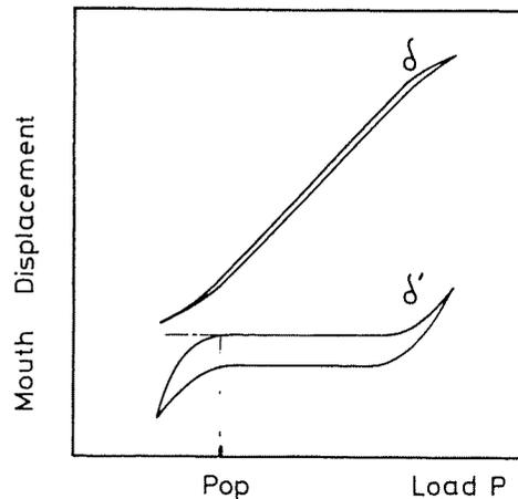
Fig 3 Determination of the load  $P_0$  corresponding to crack opening from  $\delta$  vs  $P$  and differential  $\delta'$  vs  $P$  diagrams
