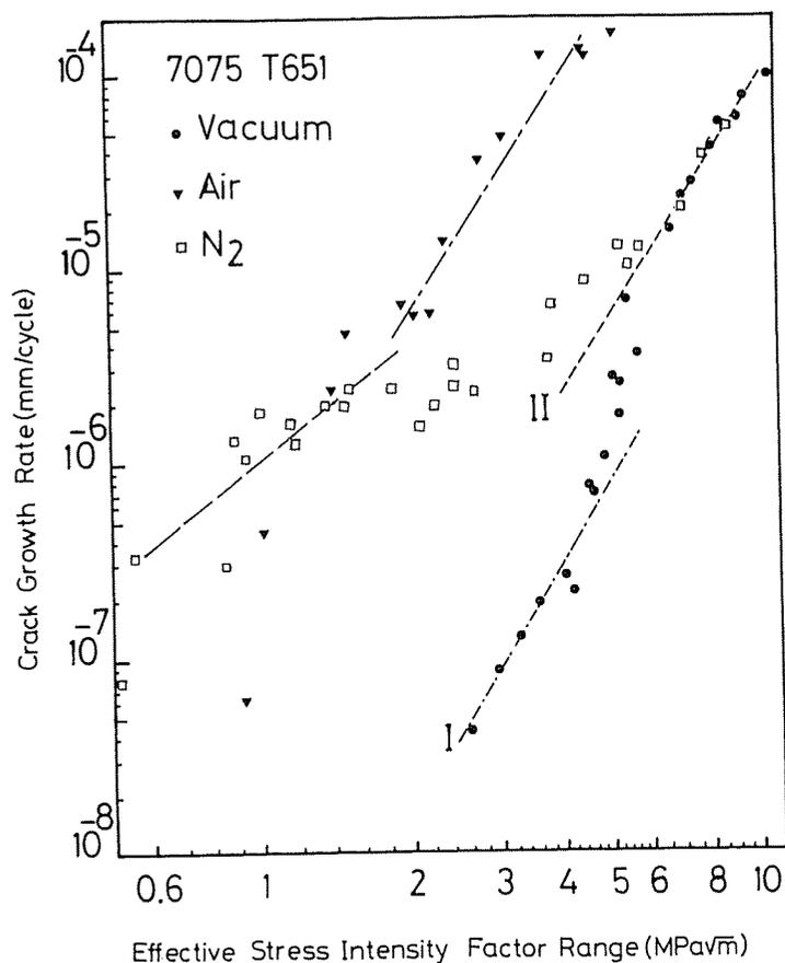
Fig 10 Crack growth rate versus  $\Delta K_{\text{eff}}$  for long cracks on the 7075 T651 alloy in air, vacuum, and nitrogen (3 ppm  $\text{H}_2\text{O}$ )
