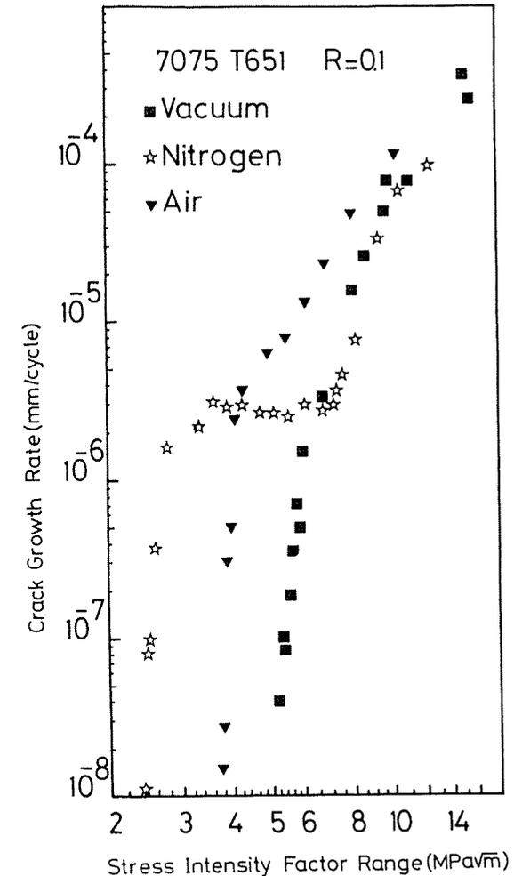
Fig 2 Crack growth rate versus  $\Delta K$  for long cracks in the 7075 T651 alloy in air, vacuum, and nitrogen (3 ppm H<sub>2</sub>O)
