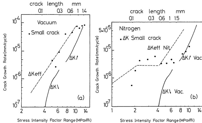
Fig 1 Crack growth rate versus  $\Delta K$  for small cracks compared with long crack behaviour in terms of  $\Delta K$  and  $\Delta K_{eff}$ .
