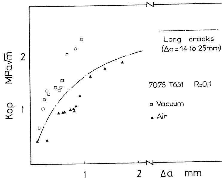
Fig 8 Variation of the opening stress intensity factor  $K_{op}$  in air and vacuum as a function of  $\Delta a$  the short crack length; 7075 T651 alloy
