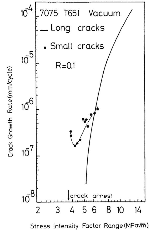
Fig 6 Crack growth rate versus  $\Delta K$  in vacuum for small cracks compared with long crack behaviour in the 7075 T651 alloy
