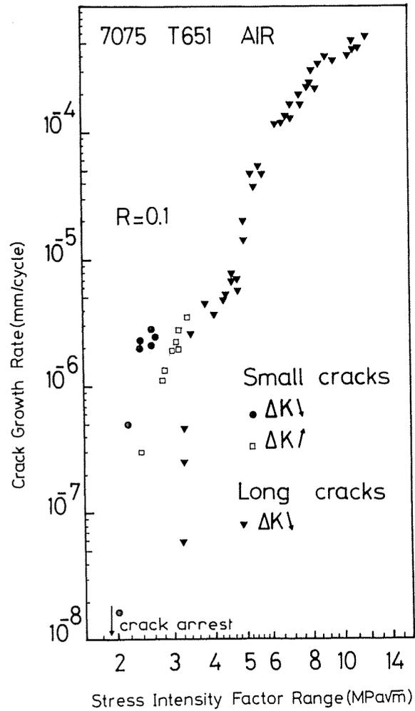
Fig 5 Crack growth rate versus  $\Delta K$  in air for small cracks compared with long crack behaviour in the 7075 T651 alloy
