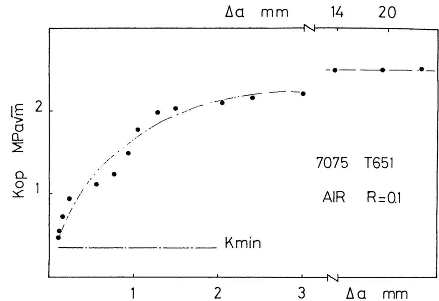
Fig 4 Variation of the opening stress intensity factor  $K_{op}$  as a function of the remaining crack length  $\Delta a$  after machining of the crack wake on the 7075 T651 alloy
