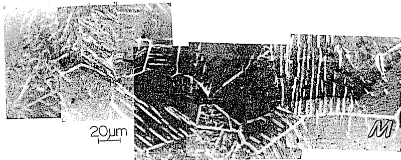
Fig 4 Early indication of the fatigue sub-surface crack appearing on the surface of the hydrogenated and outgassed sample at 49 per cent of its fatigue life. Unetched
