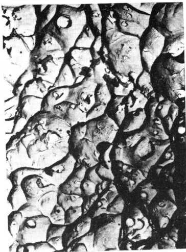
Figure 3 Ductile appearance of impact specimen fracture surface (4700:1).
