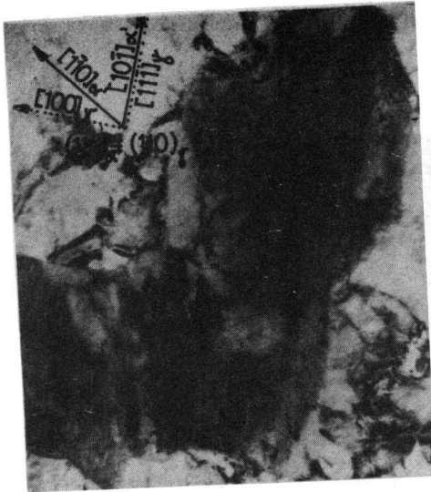
Fig. 3. The M-A constituent in underbead zone of HT 80 steel. This foil. Transmission electron microscope.
