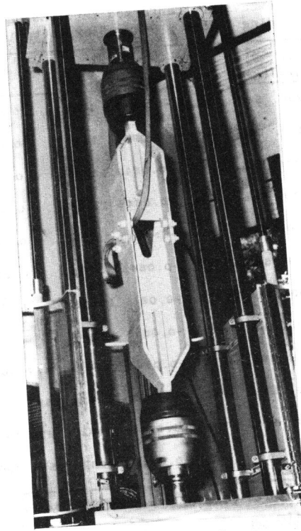
Fig. 1 Extra long frame for 1000 kN load
