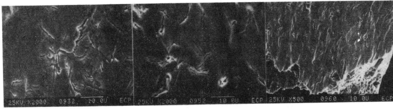
1 2 3 Collage 1.1 : recrystallized state, 275 ppm H, cavities at grain boundaries triple nodes and voids due to perpendicular hydrides
