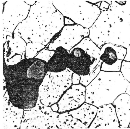
Fig.3 Crack tip region associated with fibrous crack growth in free cutting mild steel.
