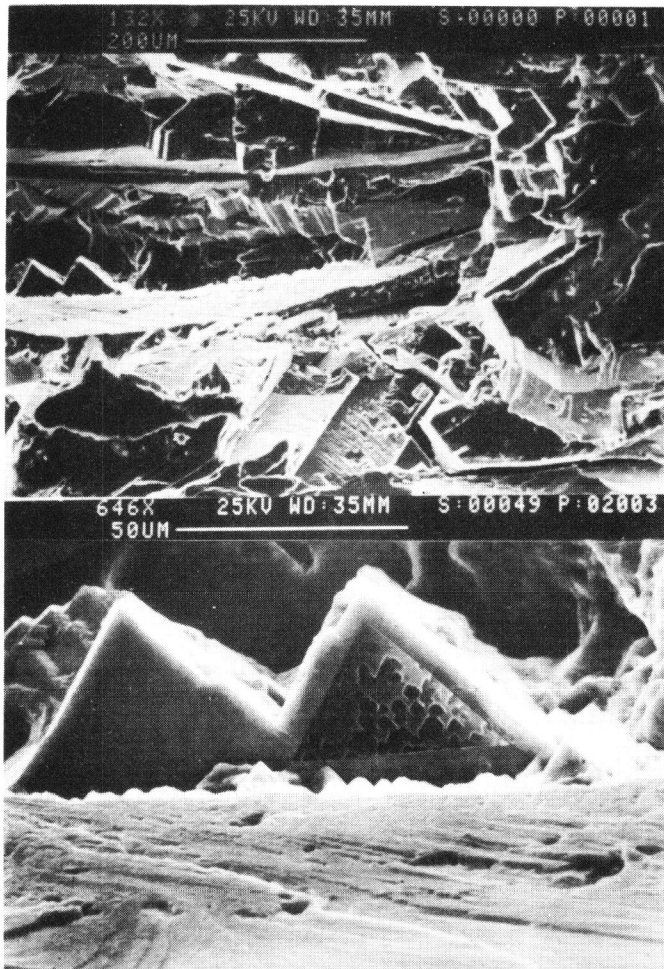
Figure 4 - a) stage I type fracture surface morphologie of the 2024 T351 alloy tested in vacuum : da/dN = 2.10^{-11} m/cycle, R = 0.5 . b) Etch-pit identification of \{111\} geometrical facets.
