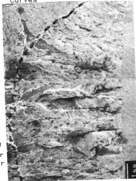
Figure 4 Brittle Fracture Surface of Specimen SSR1
