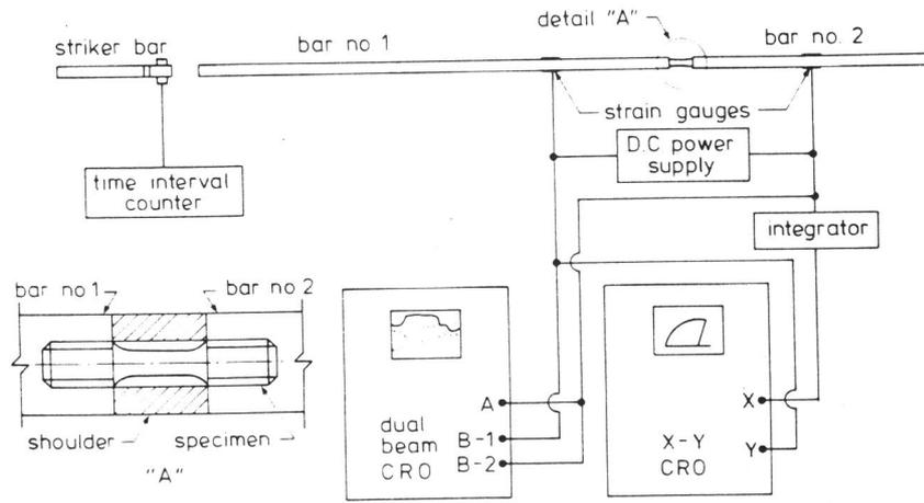
Figure 1: Tensile Test Arrangement of the Split Hopkinson Pressure Bar
