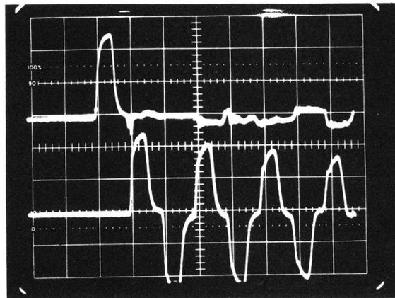
Figure 2: Typical Record of Incident and Reflected Waves
