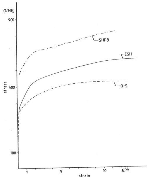
Figure 3: Dynamic and Static Stress Strain Curves for En 5K Steel
