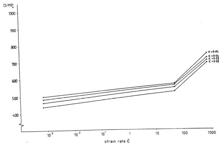
Figure 4: Strain Rate Sensitivity of Flow Stress for En 5K Steel
