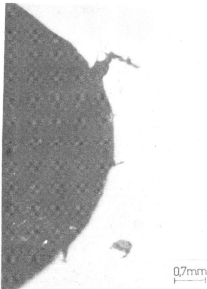
Figure 7 Nucleated microcracks at the notch tip
