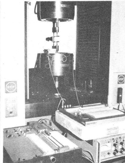
Figure 4 Experimental set-up for measurement of K_{Ic}
