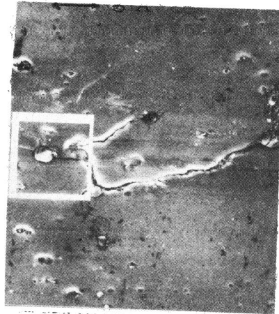
Figure 3 SEM photograph of microcracks emanated from inclusions in 2024-T4 specimen. 6580 cycles at stress amplitude = \pm 370 MPa.
