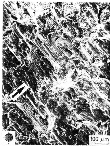
Fig. 7 Rubbing marks on fatigue fracture surface of steel 1
