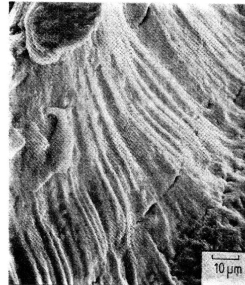
Fig. 9: Detail from Fig. 8 of Fracture Close to Origin
