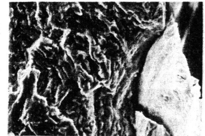
Fig. 8: magn. 1000 X. Intergranular crack initiation of fatigue fracture of controlled forged rod.
