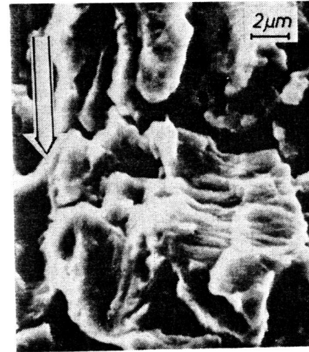
Fig. 7 SEM photograph of fracture surface at \Delta K=37 \text{ MPa}\sqrt{\text{m}} (crack growth direction is indicated by arrow).
