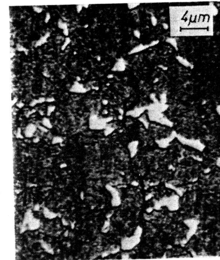
Fig. 8 Crack path observed by optical microscope near threshold level ( \Delta K \approx 15 \text{ MPa}\sqrt{\text{m}} ). In this microphotograph white and black area are martensite and ferrite respectively.
