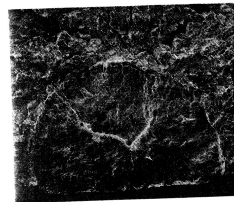
Fig. 7: closed crack front around the inclusion
