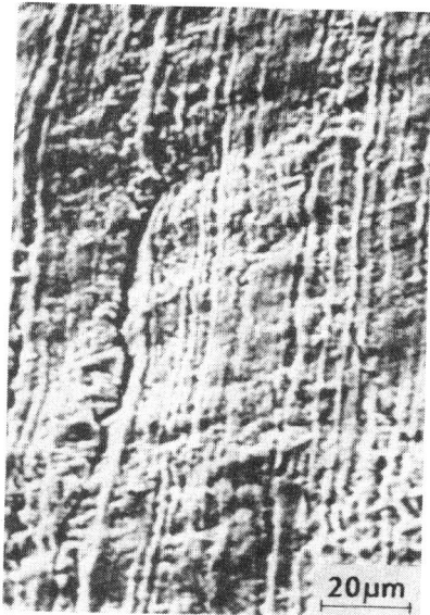
Fig.6a Oxidation of PSB's (20% PCW, 923 K, \frac{\Delta\epsilon_t}{2} = 0.25\% )
