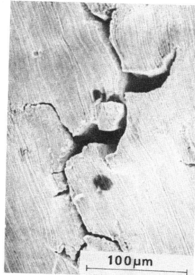
Fig.6b Grain boundary cracks at ridges (20% PCW, \frac{\Delta\epsilon_t}{2} = 0.6\% )
