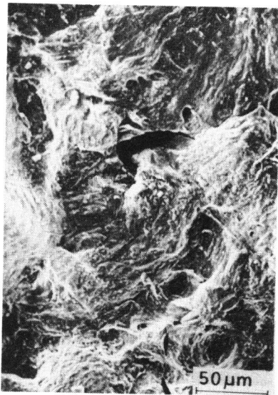
Fig.6c Fracture surface of 20% PCW (923 K, \frac{\Delta\epsilon_t}{2} = 0.6\% )
