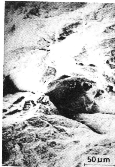
Fig.6d Fracture surface of 10% PCW (923 K, \frac{\Delta\epsilon_t}{2} = 0.6\% )
