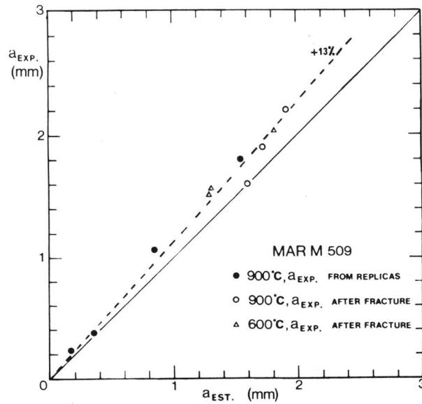
Figure 1 - Comparison of calculated ( $a_{est}$ ) and experimental ( $a_{exp}$ ) cracks depth on specimen, for several test conditions.
