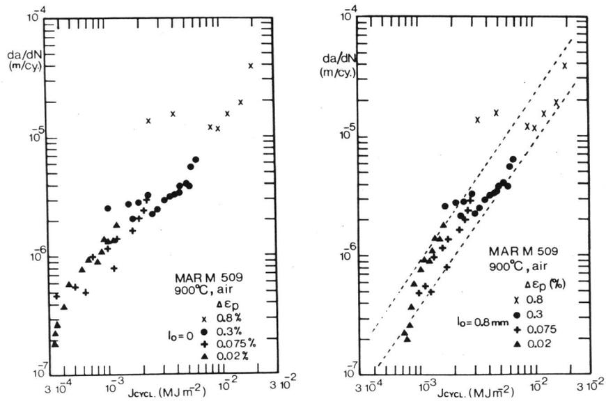
Figure 2 (left) and 3 (right) - Variation of crack growth rates as a function of  $J_{cycl}$  for various strain levels -  $l_0 = 0$  (left),  $l_0 = 0.8$  mm (right)
