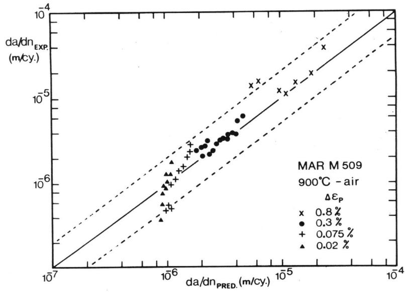
Figure 5 - Comparison of experimental ( $da/dN_{exp}$ ) and predicted ( $da/dN_{pred}$ ) crack growth rates, in air.
