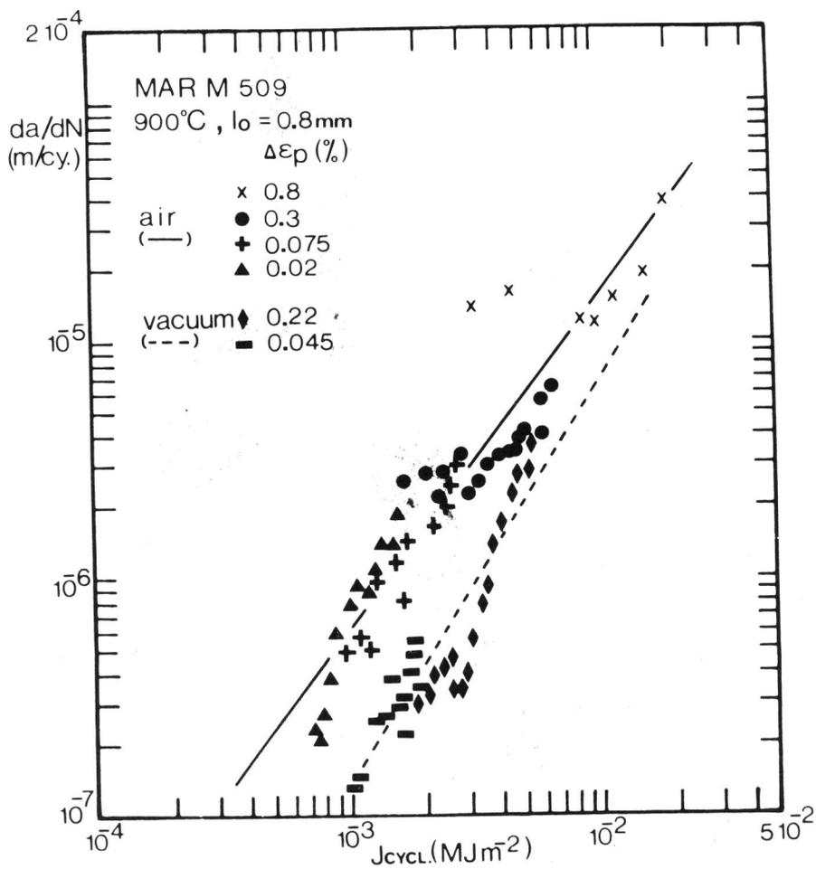
Figure 4 - Variation of crack growth rates as a function of  $J_{cycl}$  for various strain levels : comparison between results in air and in vacuum - ( $l_0 = 0.8 \text{ mm}$ ).
