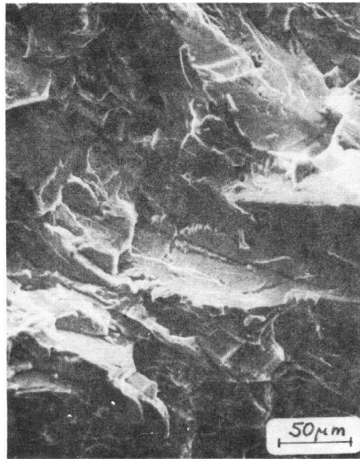
Figure 3 UA specimen in vacuum da/dN \approx 3 \cdot 10^{-6} mm/cycle
