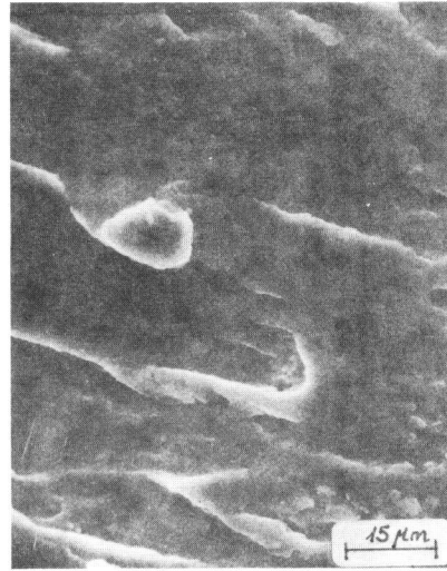
Figure 4 HOA specimen in vacuum da/dN \approx 2 \cdot 10^{-6} mm/cycle.
