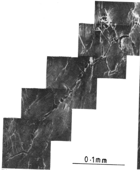
Figure 10 Fatigue crack showing intergranular and transgranular paths
