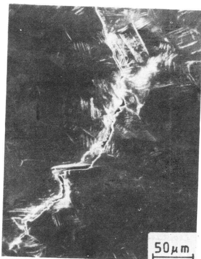
Figure 3 Microcrack in PSB air, 2 \cdot 10^6 cycles.
