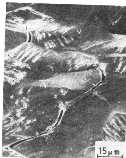
Figure 4 Grain boundary microcracks-vacuum, 4.3 \cdot 10^6 cycles.
