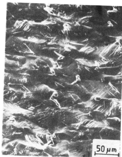
Figure 4 Grain boundary microcracks-vacuum, 4.3 \cdot 10^6 cycles.
