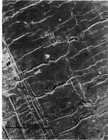
Figure 2 Shear instability cracks in 3 o'clock position of hole, formed at a nominal strain of 0.8 %.
