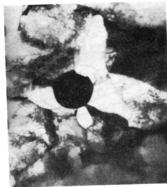
Fig. 12 : Fine ferrite grains apparently nucleated at oxide inclusions - 48 \times 10^{-3} \% O_2 :
