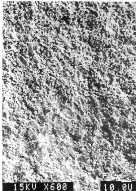
Figure 4 Transition region inter- to transgranular crack growth
